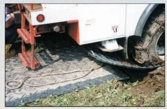
Driver called for help. AlturnaMATS were brought to the scene and tied to the chains. By putting the vehicle in reverse, the MATS were drawn under the wheels. A second MAT was placed behind the wheels enabling the vehicle to back out easily.
